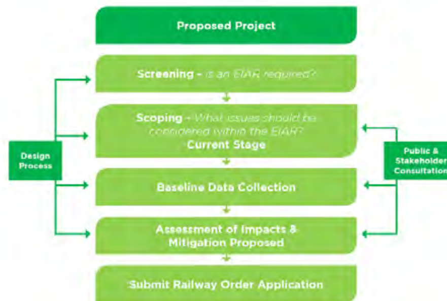
The EIA Process leading to submission of Railway Order to An Bord Pleanála
